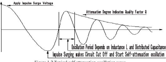
Figure 1-2 Typical self-attenuation oscillation wave
