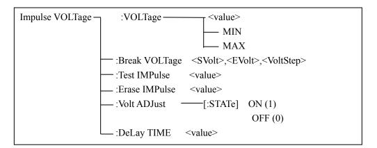
Figure 8-6 Impulse VOLTage subsystem command tree
