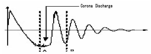
Figure 2-3 Corona Discharge Comparison
