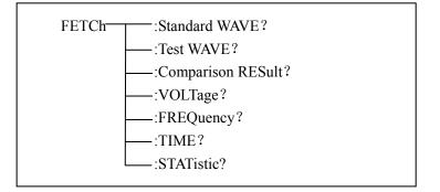
Figure 8-11 FETCh? subsystem command tree
