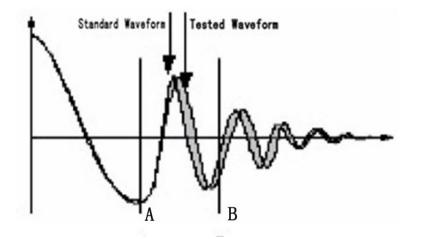
Figure 2-2 Differential Area Comparison
