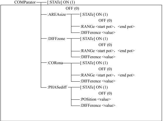
Figure 8-5 COMParator subsystem command tree
