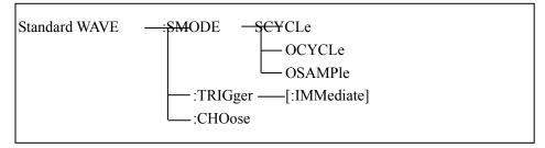
Figure 8-8 Standard WAVE subsystem command tree
